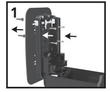
Install the TRUE FIT wall plate at the designated anchor holes. Place the TRUE FIT wall plate between the dispenser and the wall during installation.
