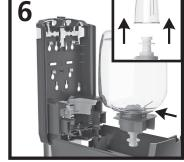
Remove refill cap and push the new refill into dispenser.
