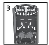
Using the dispenser, pierce the tape on the back plate to mark and drill four holes using 1/4" drill bit. Use four #10 x 1" wall anchors and four #10 x 1" screws to secure the dispenser in place, being careful not to over tighten. It is recommended to use 4 screws. If only two are possible, the top two holes should be used. **Recommended holes shown.**
