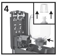
Remove refill cap and push the new refill into dispenser.
