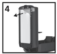
Clean installation surface with an alcohol pad. Allow surface to dry for 60 seconds then peel paper off installation tape and press the dispenser firmly against the wall for 10 seconds. For maximum adhesion, wait 24 hours before loading refill or using dispenser.
